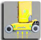
Automatic Pothole Protection
